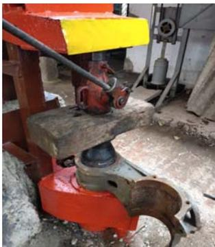
2. Local bush fitting cum removal device prepared in coaching depot muv. Now bushes of control arm and other link of LHB coaches can be assembled and disassembled in depot it self thus saving time.
