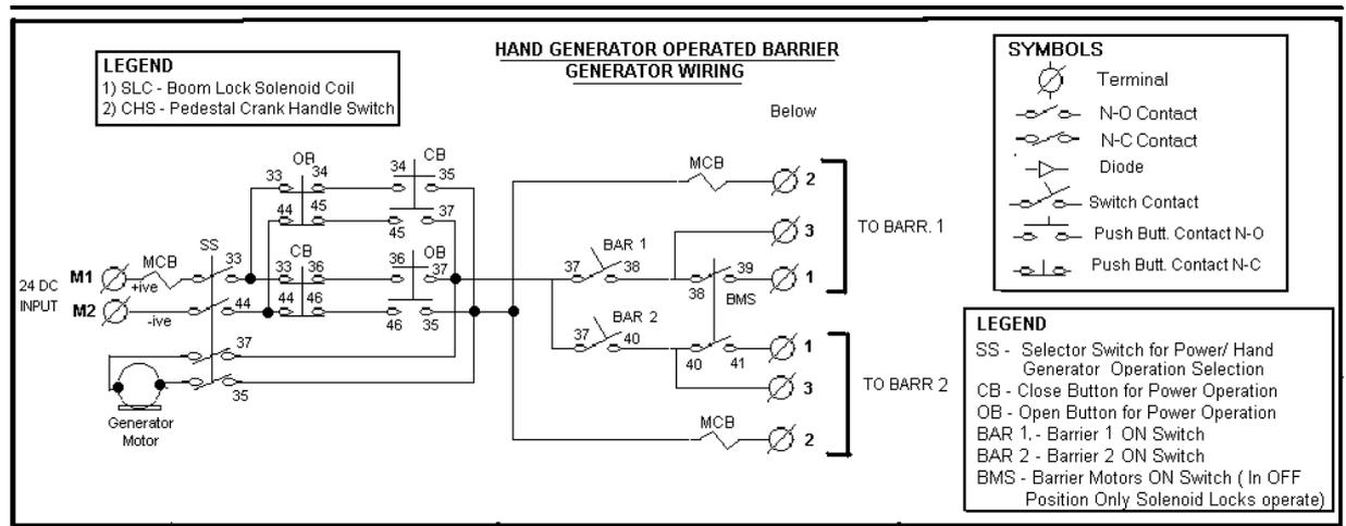
Fig.. Wiring inside the control panel
