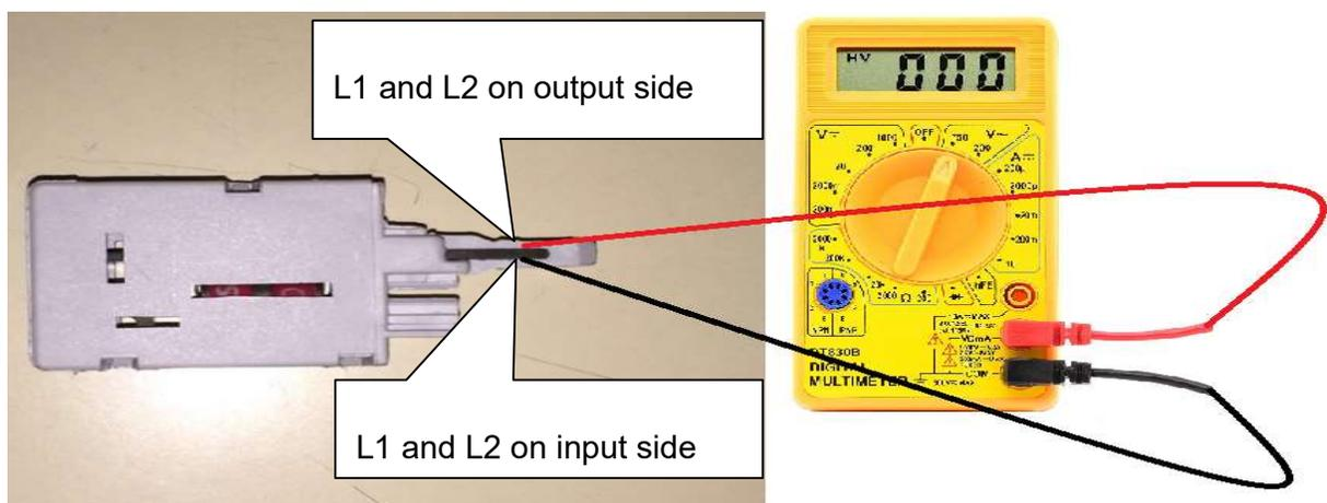
3. If continuity is there between exchange side and line side for both L1 and L2, it means PTC Resistor is working, insert the IPM back into the Krone module else replace it with a new one.
