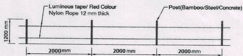
Elevation of Barricading
