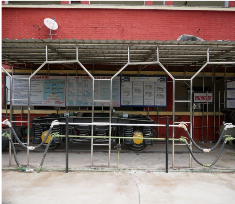
ICF Trolley with Twin Pipe Air Brake System
