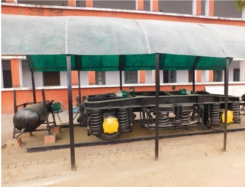
ICF Trolley with Twine Pipe Air Brake System
